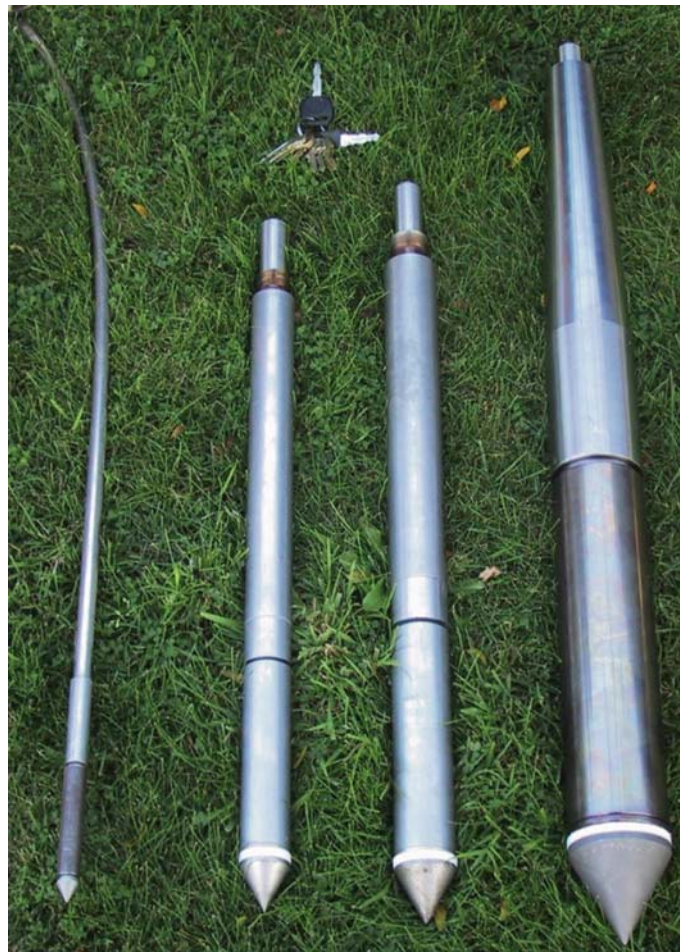
Figure 8 Range of CPT probes (from left: 2 cm 2 , 10 cm 2 , 15 cm 2 , 40 cm 2 )
