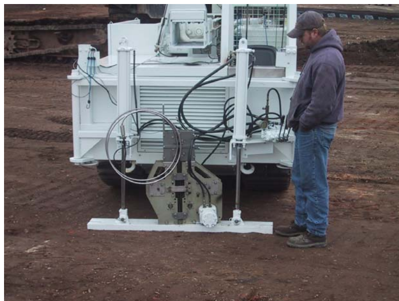
Figure 14 Mini-CPT system attached to small track mounted auger rig
