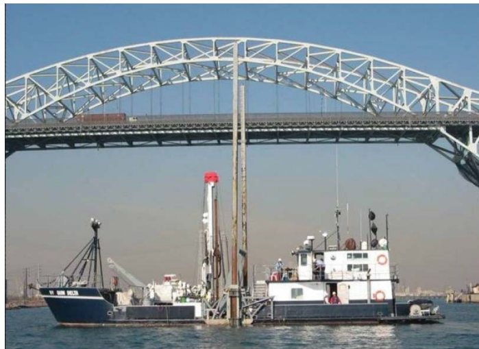
Figure 16 Quinn Delta (Gregg) ship with spuds
