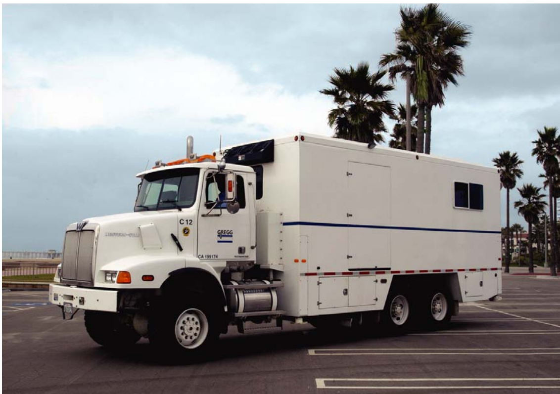
Figure 10 Truck mounted 25 ton CPT unit
