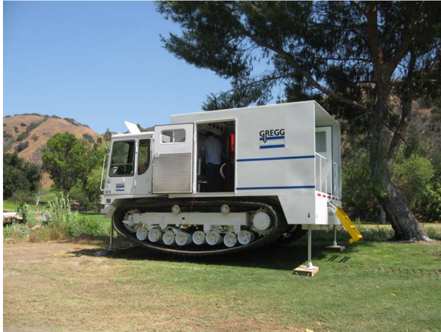
Figure 11 Track mounted 20 ton CPT unit
