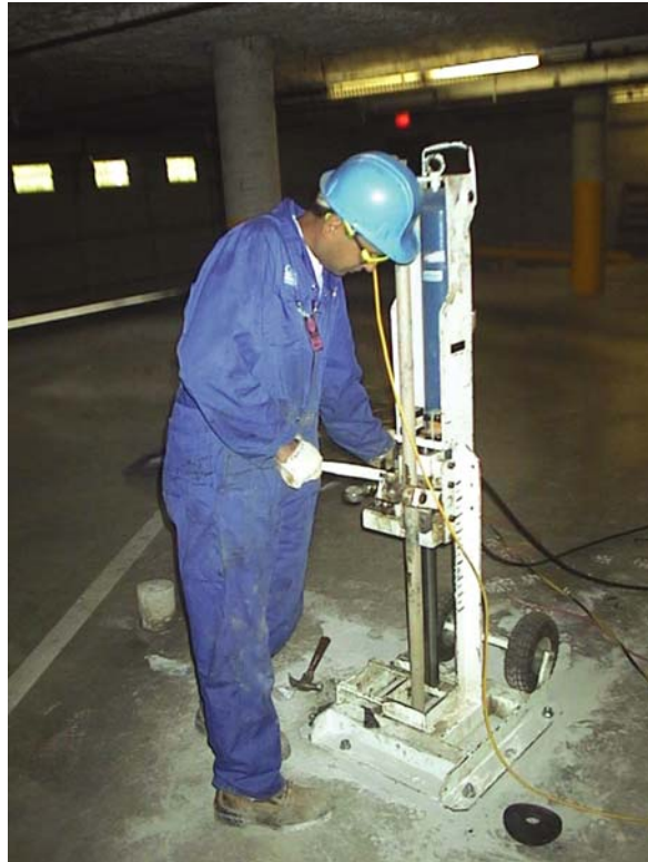
Figure 13 Portable ramset for CPT inside buildings or limited access
